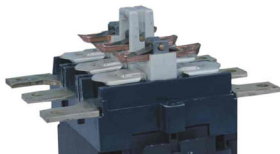
8. Contact systems of products above 370A adopt mechanism with arc isolation contacts and conductive contacts.
